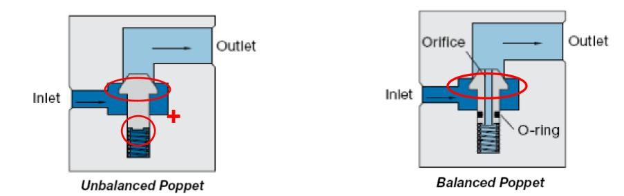
**Balancing reduces the area on which P**<sub>inlet</sub> acts.
