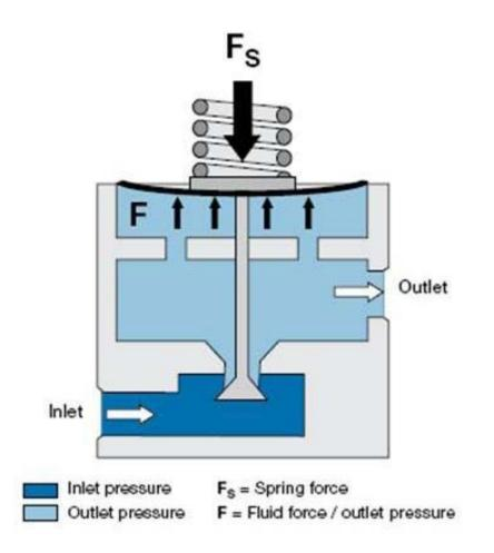
The function of a pressure reducing regulator is to reduce a pressure and to keep this pressure as constant as possible while the inlet pressure and the flow may vary.
